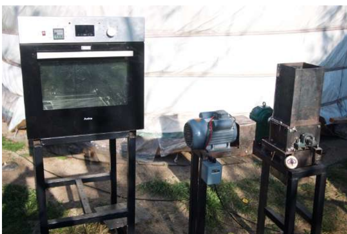
Ecosoum's home-made plastic recycling machines
